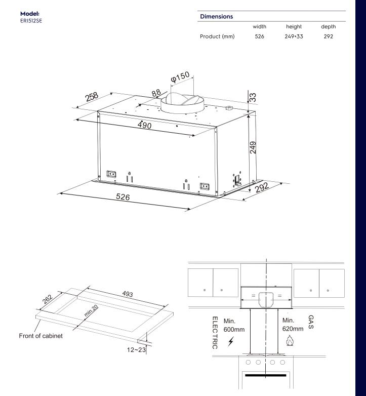
Please note! Dimensions to be used as a guide only. All customers MUST refer to the user manual supplied with the product for detailed installation instructions. © 2023 Electrolux S.E.A PTE. LTD. ELX\_DIM\_ERI512SE\_Nov23
