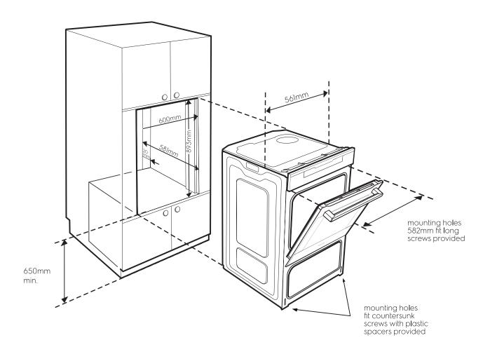
\*D - Dimension For proper ventilation there must be a gap at the bottom rear of the cabinet. This can be a slot 20mm deep or an equivalent, full width opening (e.g. a series of holes) with a min area of 120cm<sup>2</sup>. The opening must be clear of the product when fully installed. This is a requirement of any EVExxxxxx and Duo models. If the supply cord is damaged it must be replaced by the manufacturer, its service agent or similarly qualified persons in order to avoid a hazard.
