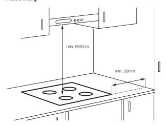
NOTE: The clearance must meet or exceed the minimum recommended for both the rangehood and cooktop. Refer to the rangehood installation manual.
