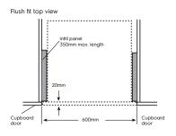
Infill panels are recessed 20mm from the external cabinet door to accommodate flush fit.
