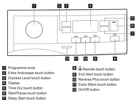
I Press the touch buttons with your finger in the area with the symbol or name of the option. Do not wear gloves when you operate the control panel. Make sure that the control panel is always clean and dry.
