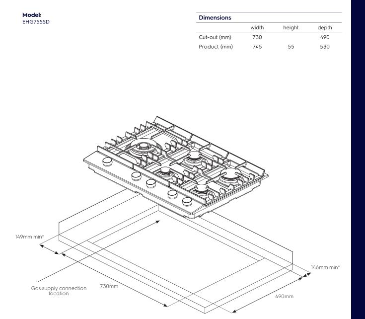
\*To combustible surface (dimension is not relevant if the adjacent surface is non-combustible).
