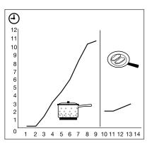
You can get a necessary heat setting in a shorter time if you activate the Automatic Heat Up function. This function sets the highest heat setting for some time (see the graphic), and then decreases to the necessary heat setting. To start the Automatic Heat Up function for a cooking zone:
