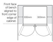
When positioned in a corner area, spacing of at least 300mm on the hinge side will allow the doors to open enough to enable the removal of bins and shelves.
