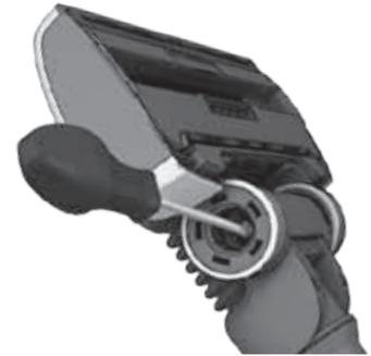
Unscrew the wheel axis and clean all parts. Refit in reverse order.
