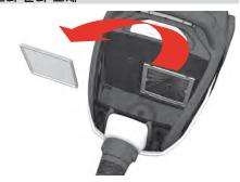
Pull the grip and remove the filter frame. Remove / Clean the filter Re-assemble filter holder by placing back in the lower part and put the frame in place at the top.
