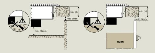
WARNING: Under no circumstances should the cooktop base be installed directly onto a shelf.
