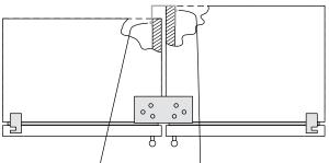
Two cabinets of different depths joined at the back with rear clamp. Notice that compressor mounting plate fasteners are in different location on the rear clamp.
