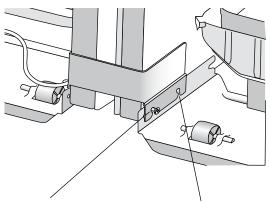
Leave the compressor mounting plate fastener partially loose after engaging the rear bracket. This hole on the rear bracket is used only when two cabinets of different depths (D1) are being joined together (i.e. 690 + 595 model or 790 + 595 model).
