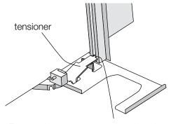
Engage the center cover piece into the tensioner of the bottom bracket. To facilitate this loosen the tensioner if required.
