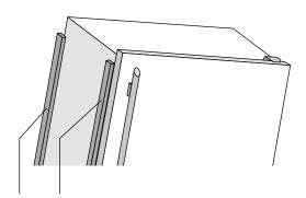
Secure protective foam to the side of the cabinet using tape supplied in the connection kit. Foam should be secured on the handle side of the cabinet.
