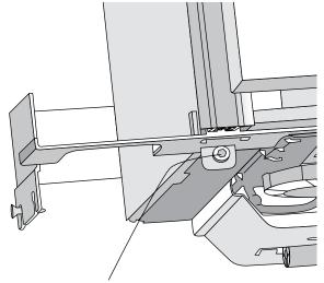
Tension on the center cover can be adjusted with the screw on the bottom bracket
