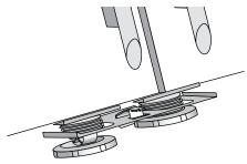
7. With the two cabinets provisionally connected level both units using adjustable rollers as per recommendations in your owner's manual. Gently push the assembly back into the wall cavity and check for alignment and level. If necessary, pull the cabinets out again and adjust, repeat the procedure until satisfied with level and alignment.
