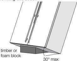
Tilt the cabinet back by no more then 30 degrees. This will enable adequate access to the front feet in order to install lower bracket. Ensure that assistant has firm grip of the cabinets before continuing. Use chocks or other means of firmly supporting the cabinets before attempting further installation work. The cabinets can be best tilted by having assistant pull and support the appliances from the back.
