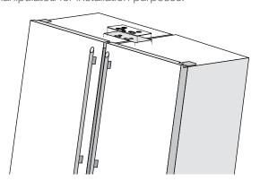
4. Provisionally join the two cabinets together at the back, near the compressor, using the rear clamp. Loosen the fasteners connecting the compressor mounting plate to the cabinet and engage rear clamp, leave the fasteners partially loose at this stage.
