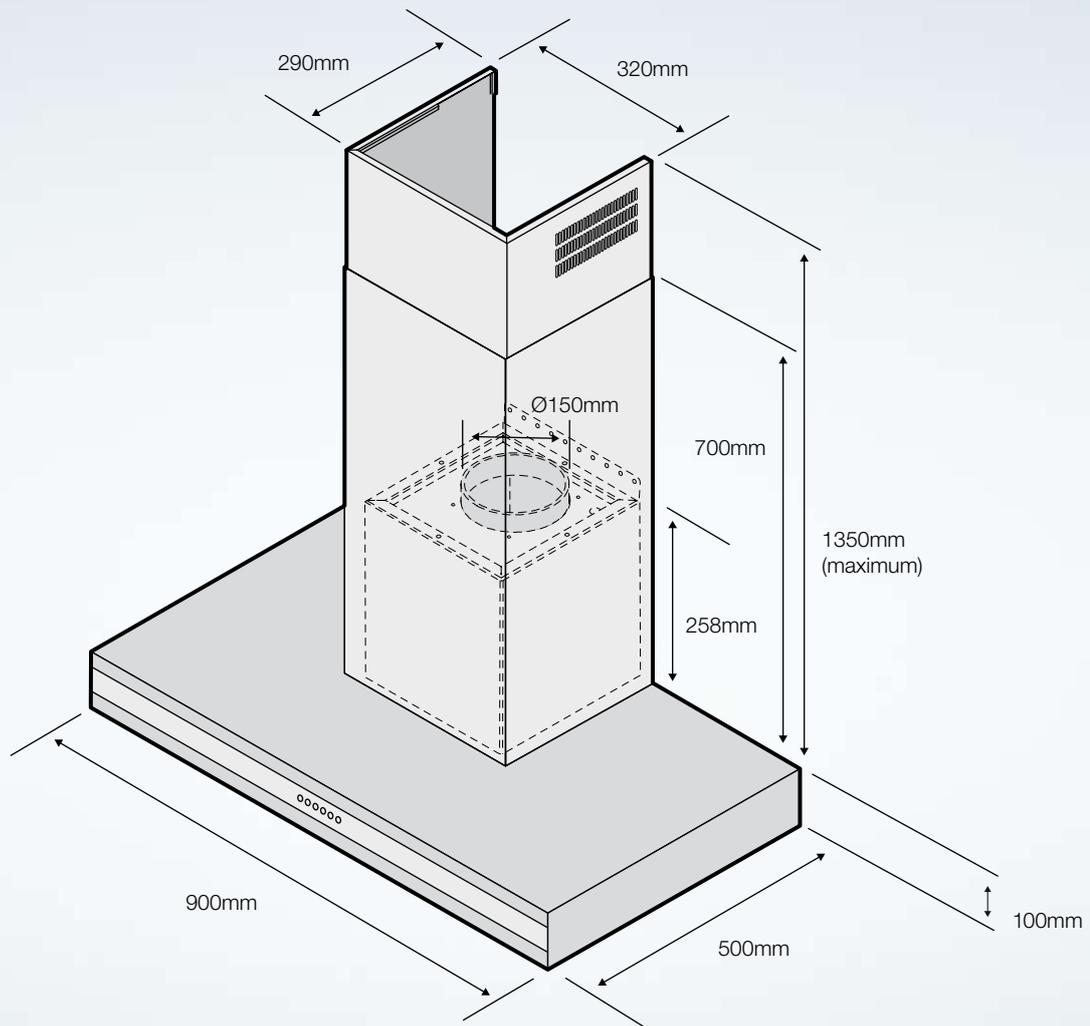
**Note:** This is a guide only. It should not be used for installation specifications. Refer to owner's manual for full installation information.
